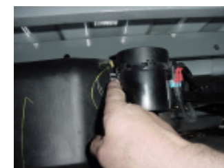
Step 2: Disengage the locking pin.
