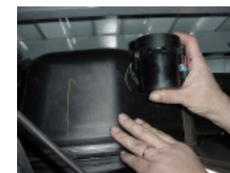
Step 3: Slide fuel valve from bracket.
