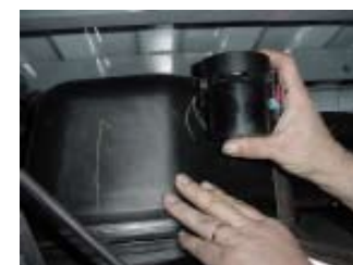
Step 3: Slide fuel valve from bracket.
